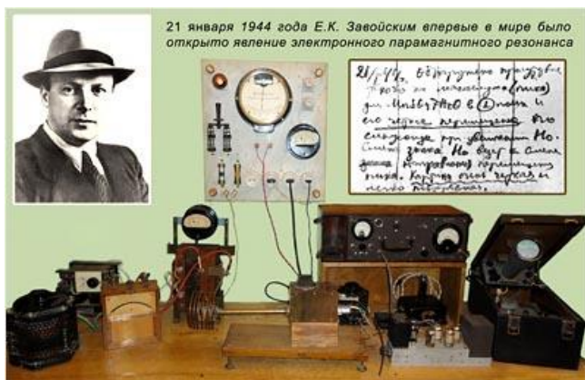
Fig. 4. Zavoisky's experimental set to study the electron paramagnetic resonance.
